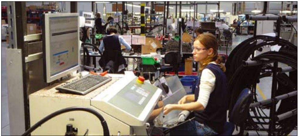
Schleuniger PowerStrip 9500 for jumper production
