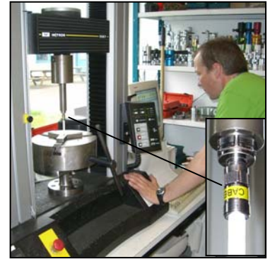
Computer controlled test of the pull strength
