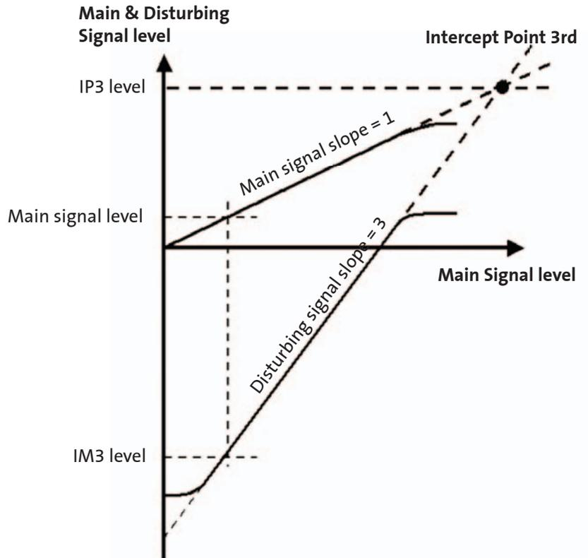
The IP3 (Intercept Point 3<sup>rd</sup>) measured in dBm. IP3 is the fictive point where the two signals meet, if one imagines that the main signal strengthens until the two signals come together as shown on the illustration.
