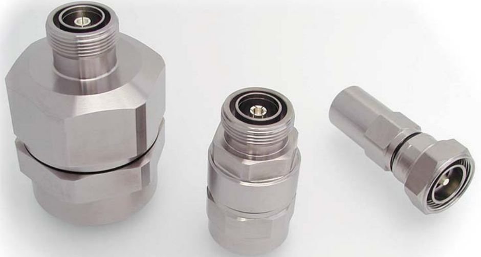
50 ohm connector examples, from left: 7/16 F for 1-5/8" Annular cable, 7/16 F for 7/8" Annular cable & 7/16 M for 1/2" Superflex cable
