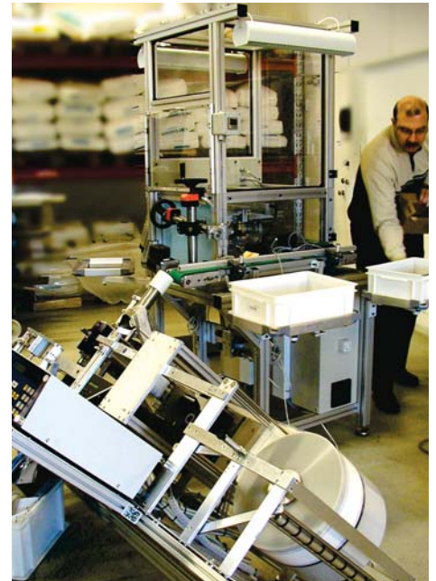
The new packaging machine under construction and test.
