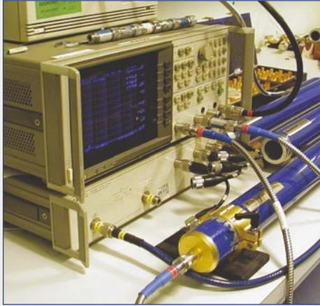
*The CoMeT set-up for measurements of screening efficiency and transfer impedance.*
