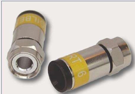
*The UltraEase™ body is made of black UV resistant polymer and the post is made of C 36000 Brass Alloy.*
